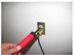
Air moves through these outlets which have no direct connection to the outside. This demonstrates that air moves freely through the unsealed fiberglass, which allows cold air to enter and warm air to escape to the attic.
