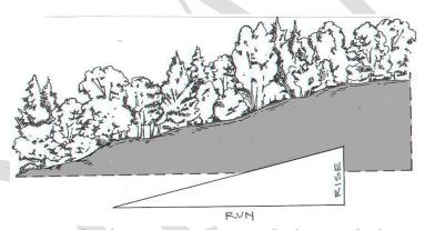
Slope, or gradient, is measured as the increase in rise over run. In this example, the rise increases (climbs) 15 feet over a distance (run) of 100 feet, which results in a 15% slope.
